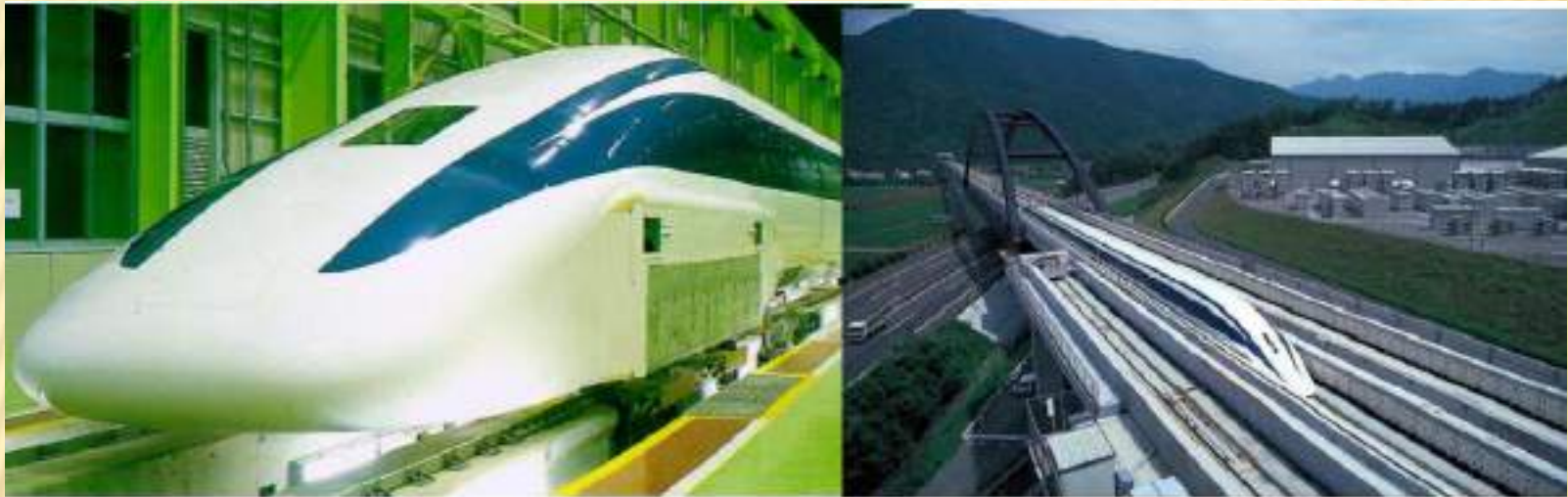
Miyazaki Maglev (Japan) Test Track, 40 km
