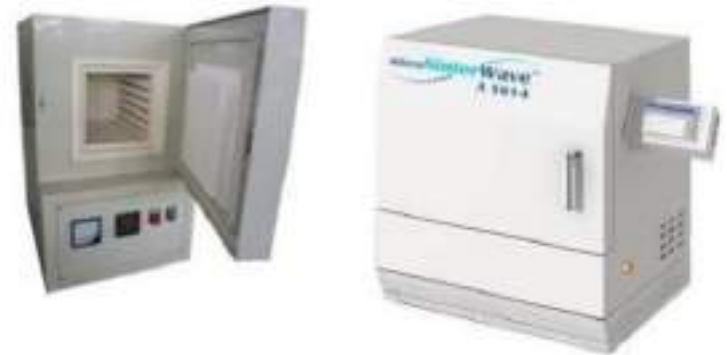
Simple microwave ovens used in microwave sintering
