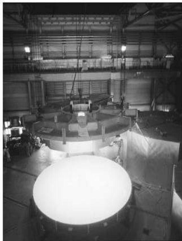
Figure 4.13 Processing of 8.2 m Zerodur® glass-ceramic telescope mirror.
