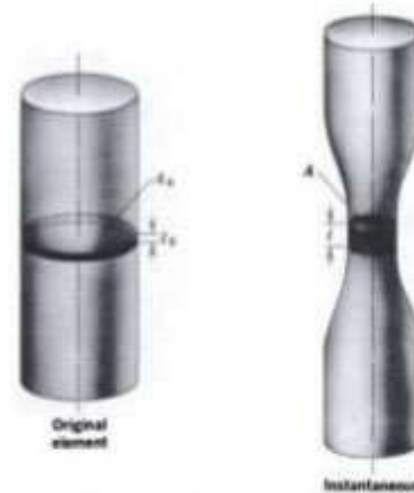
Figure 2.7 Localized plastic flow causes "necking" to occur in a tensile specimen.
